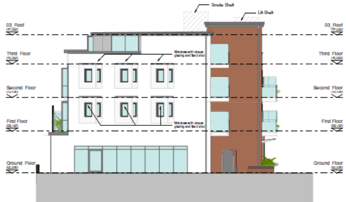
3 North West Elevation 1 : 100
